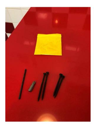
2. Lay out holes to be drilled, and drill pilot holes. For the 24"W/1PS booth, the wood panel is 17" wide. For the 48"W/2PS booth, the wood panel is 41" wide. For the 72"W/3PS booth, the wood panel is 65" wide. The post-to-post spacing (*excluding* the alignment flanges) should match the panel width exactly. DOUBLE CHECK MEASUREMENTS *BEFORE* DRILLING PILOT HOLES.
